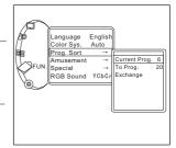
5. Press the CH+/- buttons to move the indicator to " Exchange ".
